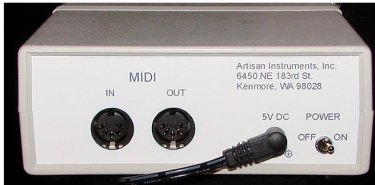
2. Connect the power supply to the power jack on the rear panel. Please note: Only use the 5 volt DC power supply that comes with your Artisan Sequencer. Using a power supply that is less regulated or the wrong polarity can destroy both the Sequencer and the USB Memory Device.
