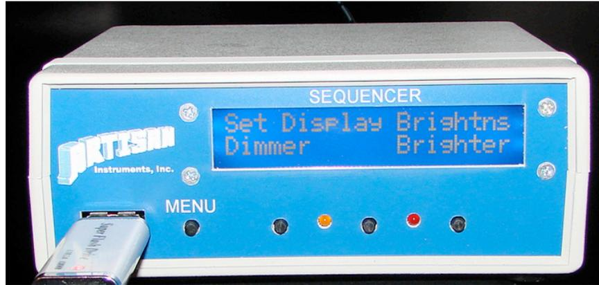
Pressing the MENU button again will bring you to the display contrast screen. Press the Lighter and Darker button to achieve the desired display contrast.
