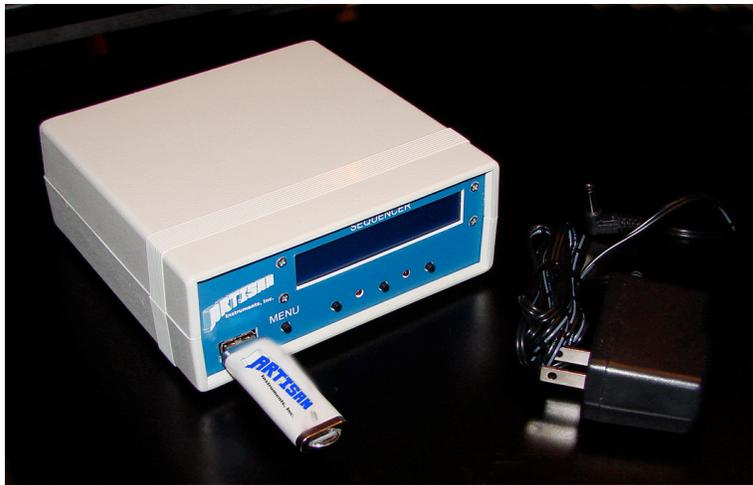
1. Unpack your Sequencer and connect the MIDI IN and MIDI OUT cables to the back panel. See addendum at the end of these instructions for information on how to properly connect your new Sequencer to your MIDI devices and/or Artisan Control System. Note the three unlabeled buttons on the front panel. When powered up the functions of those buttons will be displayed on the lower line of the LCD screen. The Menu button moves between sets of functions.
